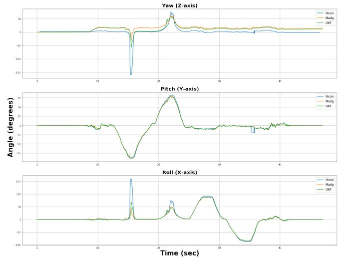
Fig. 2. Comparison of Attitude Estimation using the various filters with the Vicon Ground Truth for the second dataset.
