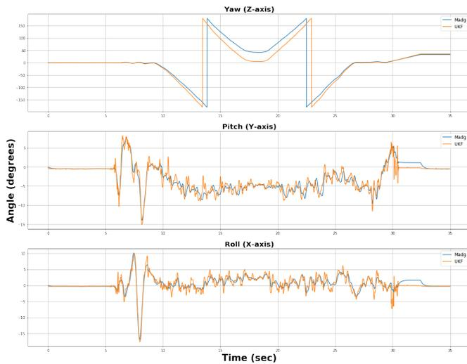
Fig. 8. Comparison of Attitude Estimation using the various filters for the eighth dataset.
