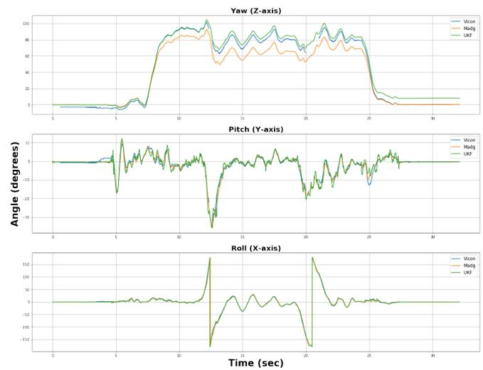
Fig. 6. Comparison of Attitude Estimation using the various filters with the Vicon Ground Truth for the sixth dataset.
