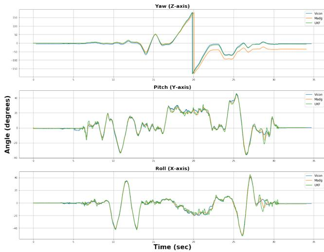
Fig. 3. Comparison of Attitude Estimation using the various filters with the Vicon Ground Truth for the third dataset.
