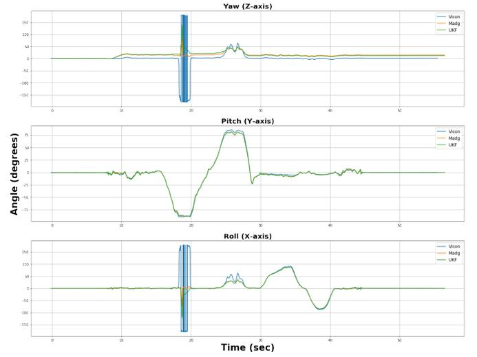
Fig. 1. Comparison of Attitude Estimation using the various filters with the Vicon Ground Truth for the first dataset.
