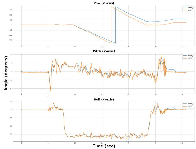
Fig. 10. Comparison of Attitude Estimation using the various filters for the tenth dataset.
