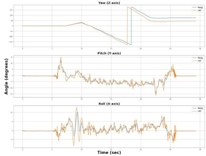
Fig. 9. Comparison of Attitude Estimation using the various filters for the ninth dataset.
