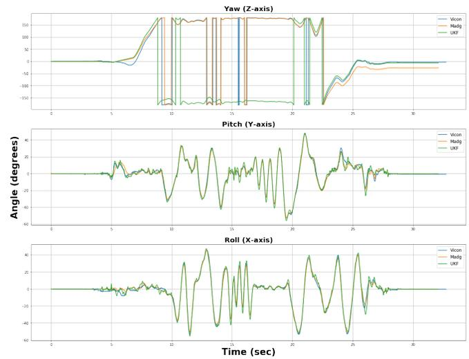
Fig. 5. Comparison of Attitude Estimation using the various filters with the Vicon Ground Truth for the fifth dataset.
