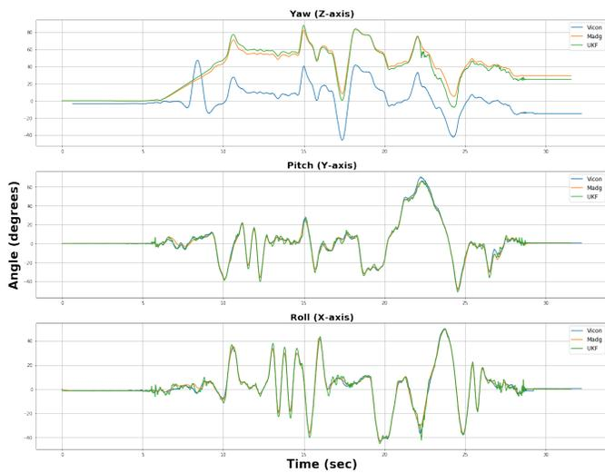
Fig. 4. Comparison of Attitude Estimation using the various filters with the Vicon Ground Truth for the fourth dataset.
