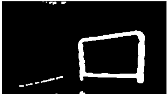
Fig. 8. Binary mask after Erosion/Dilation
