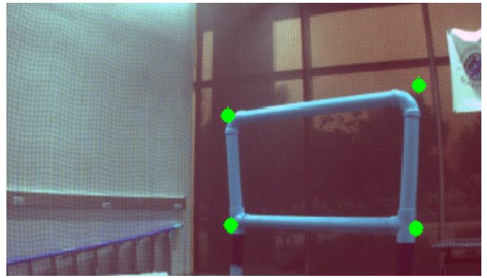
Fig. 12. Final window corners detected
