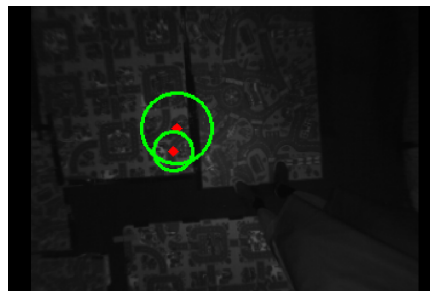
Fig. 3. Without any thresholding, HoughCircles will pick up extraneous circles.
