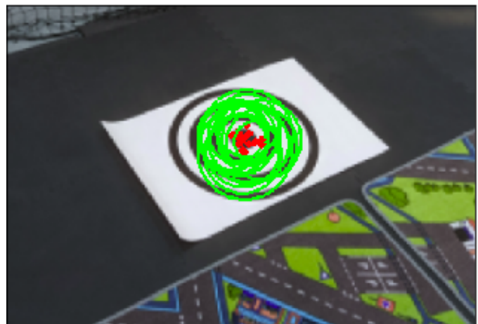
Fig. 2. Circles fitted to binary image, overlaid on original (non-Duo) image as an example. Note: Unrealistic camera orientation while in flight
