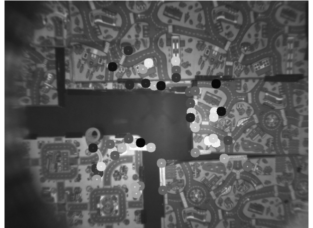
Fig. 2: Corner points detected using the KLT algorithm. Gray and black circles represent these corner points detected in the first left image of the stereo camera.
