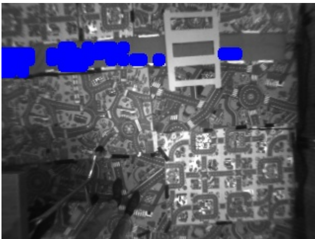
Fig. 4. Filtering the River candidates by y position (in camera frame) allows for the river to be found identified correctly.
