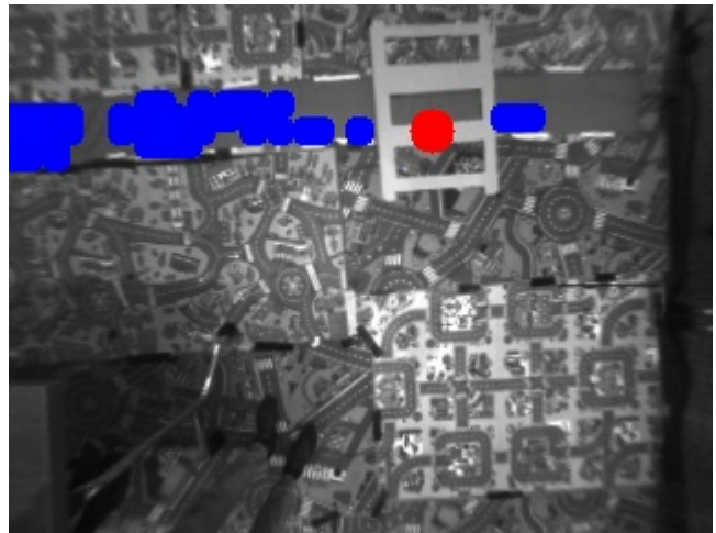
Fig. 5. The largest gap in the river is assumed to be the bridge - as long as this gap is larger than a certain threshold.
